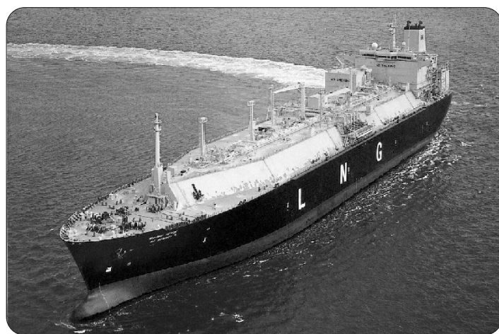
LNG is transported overseas by ship. Many of these ships have a membrane hull design.
