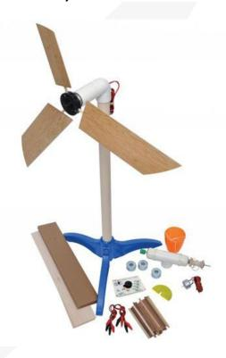
The turbine can be modified by adding an advanced wind kit gearbox to the top of the tower or by replacing the hub with a spool and string to allow the students to determine how much weight can be lifted by their blade design (not included in the basic kit).
